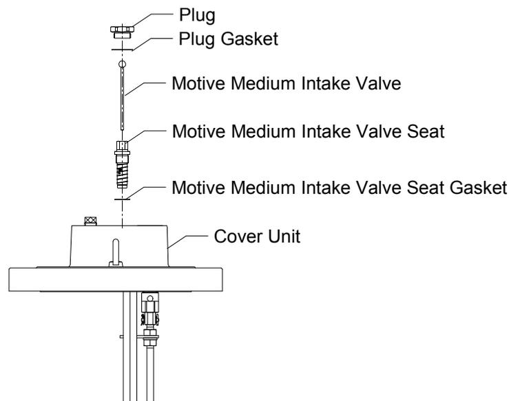
NOTE: It is possible to remove and replace the intake valve (motive medium) without first removing the cover of the PowerTrap (see instructions above).
