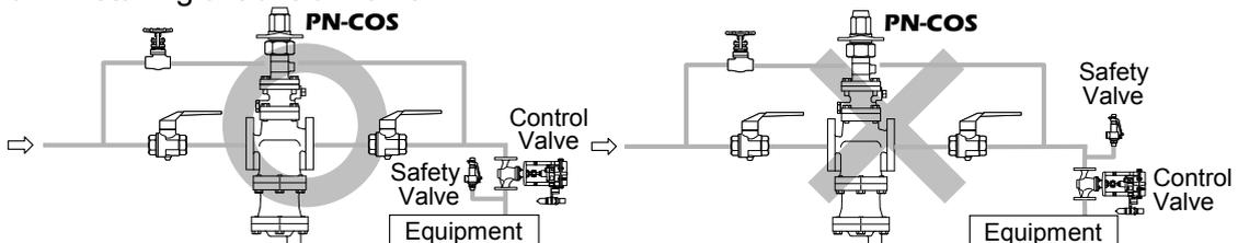
A control valve installed between the **PN-COS-16** and the steam-using equipment (downstream of the **PN-COS-16**) for controlling equipment temperature may raise the pressure between the **PN-COS-16** and the control valve when the control valve is closed, depending on the spatial relationship. A safety valve should be installed downstream of the control valve.
