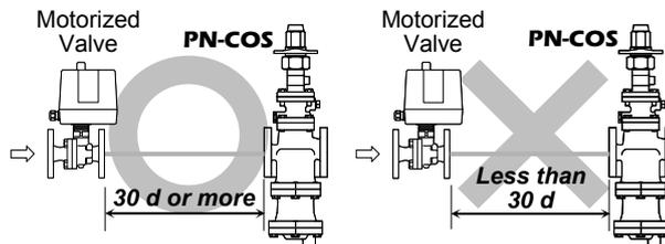
Maintain a straight piping run of **30 d or more** when a pressure reducing valve is installed.
