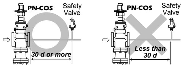
Maintain a straight piping run of **30 d or more** when a control valve or an automated valve (on-off valve) is installed.
