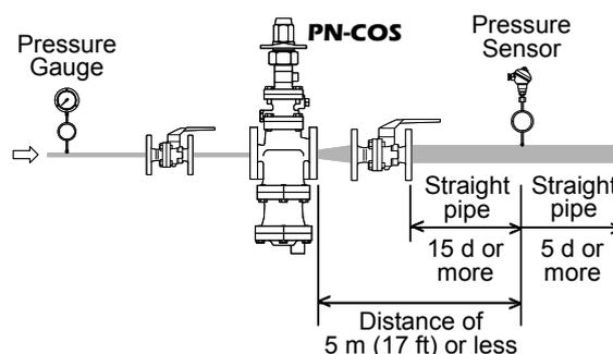
Steam fluctuations at the pressure sensor may impair the stability of the pressure control. Ensure a straight piping run of at least 15 d upstream and 5 d downstream from the pressure sensor.
