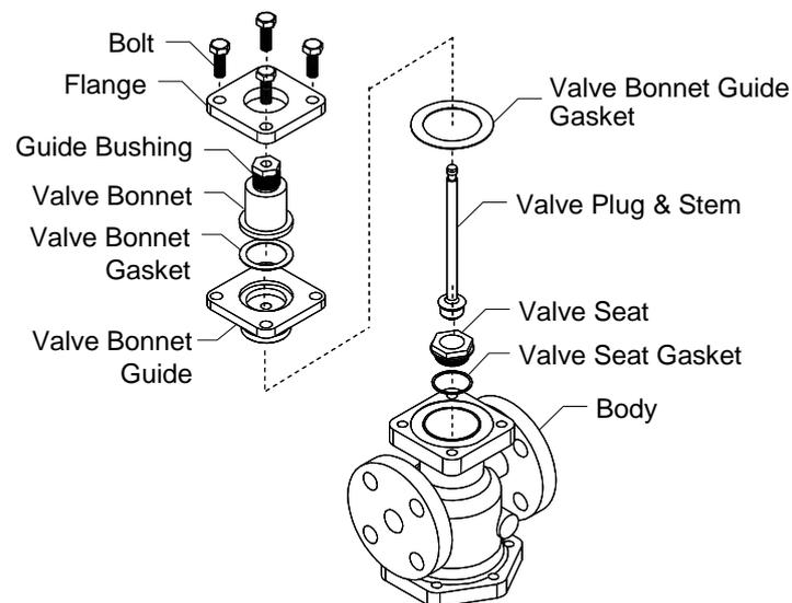
**Removing / Reattaching the Separator and its Components**
