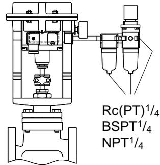
Integrated Filter: 5 µm + 0.3 µm
