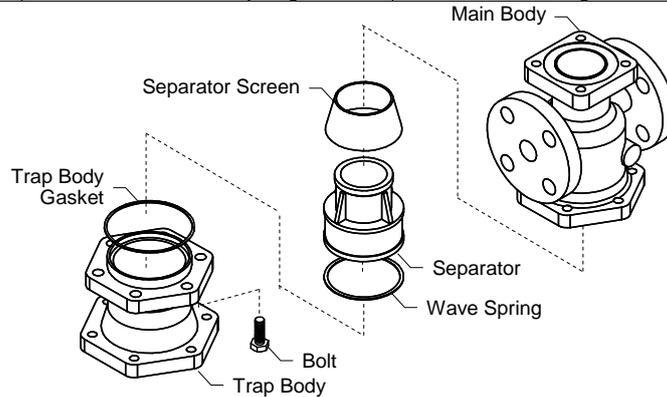
**Removing / Reattaching the Trap and its Components**
