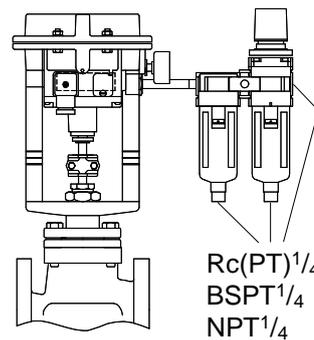
Integrated Filter: 5 µm + 0.3 µm
