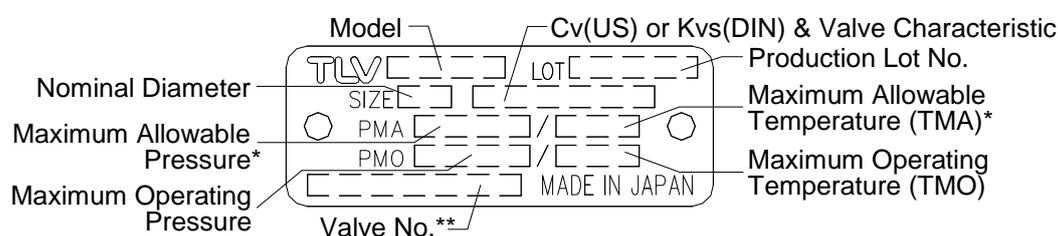
\* Maximum allowable pressure (PMA) and maximum allowable temperature (TMA) are PRESSURE SHELL DESIGN CONDITIONS, **NOT** OPERATING CONDITIONS.
