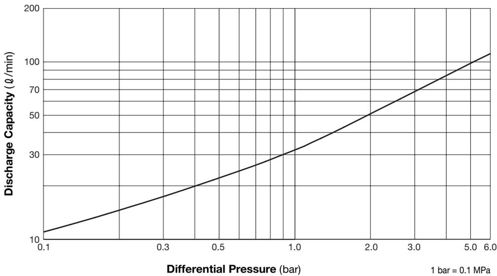
1. Differential pressure is the difference between the inlet and outlet pressure of the air vent.
