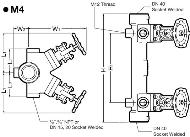
M4 is the basic manifold; SM and CM are the manifold packages combining one or more M4 units with steam traps and valves. Dimensions given here are for a single M4 manifold only. Connection types/sizes and overall length, height and weight for the SM and CM manifold packages will vary depending on the number of M4 manifolds used and the valves and steam traps installed.
