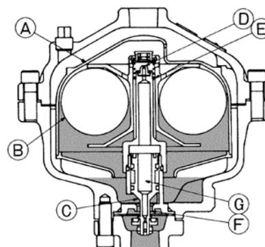
4. When the condensate has been discharged, the floats (B) fall, causing the pilot valve orifice (D) to close. When the pilot valve orifice (D) closes, the pressure in the pressure chamber (G) is released to the outlet and the piston (C) rises to close the main valve orifice (F).
