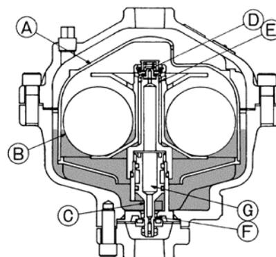
2. When the condensate level in the trap body rises to a certain point, the floats (B) rise. This, together with the help of the coil spring (E), lifts the float holder, causing the pilot valve (D) to open.
