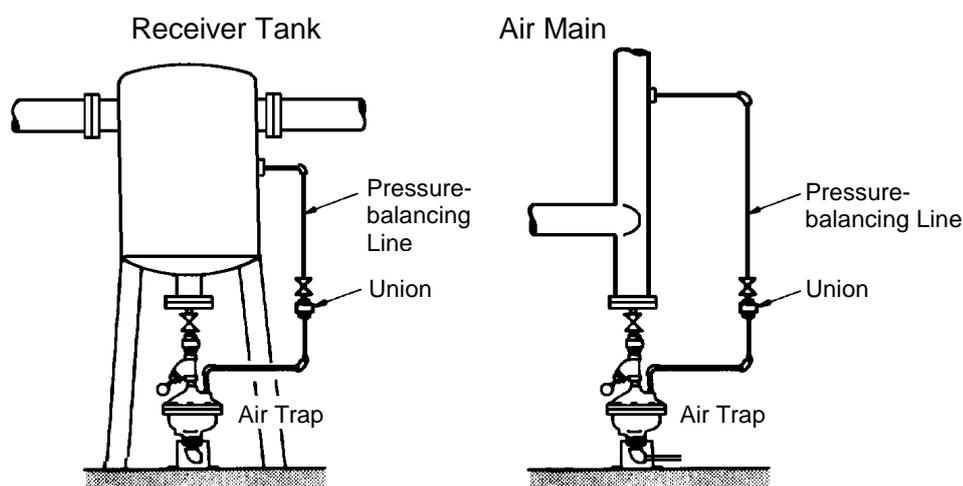
Note: Be sure to connect the pressure-balancing line to an area with the same pressure or to an air section downstream of the flow medium.
